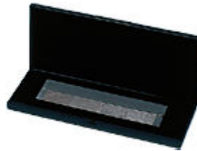
Photo: Calibration Block Type 2 in accordance with DIN EN ISO 3452-3
